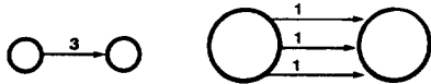
Fig. 3. Unitizing a general weighted directed graph to a unitized graph by splitting vertices.
